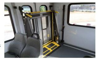
• Wheelchair Securement. Each wheelchair space is equipped with securement devices to meet the requirements of DOT 49 CFR Part 38.
